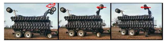
5. Lightly actuate the frame cylinders on the tractor to remove the wings from the locking system.
