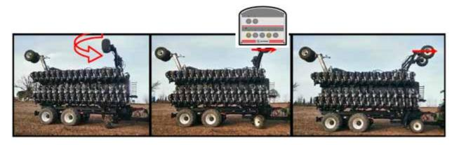
9. Lift button 2 to fold the lift assist and the side gauge wheels.
