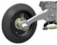
Pull the adjustment lever out to the level of the press wheel and position it on the desired notch.
