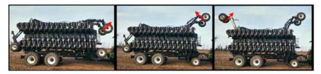
4. Lift button 4 to unfold the side gauges.
