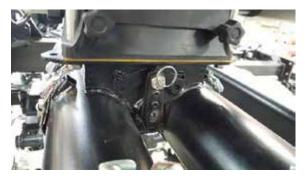
To send the contents of the hopper to all of the seed drill, the lever must be in the middle position to select one of the two rows. Position the lever on the corresponding row. Repeat this action on all the metering units.
