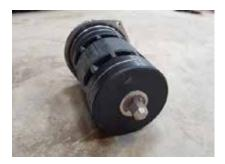
Remove the circlip holding the individual rotors to the hexagonal shaft using a hammer and a pin punch.
