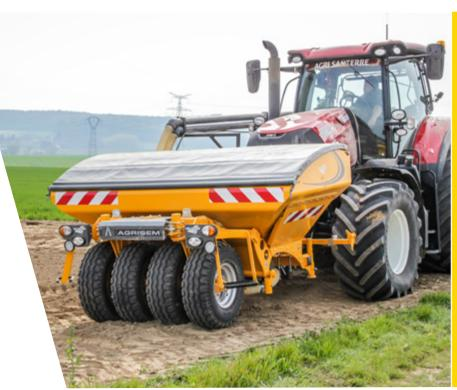
AGRISEM has developed a range of front hopper that combines with other machines.
