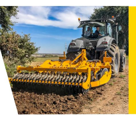
The MAXIMULCH® is a combined machine which offers the fonctions of a soil loosener and of stubble breaker.
