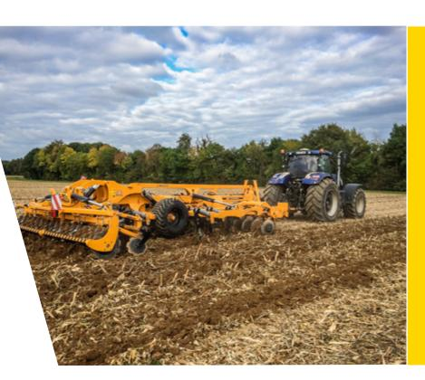
The MAXIMULCH® is a combined machine which offers the fonctions of a stubble breaker and of soil loosener.
