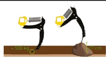
Release at the tip: +500 kg of pressureImportant clearance for the release
