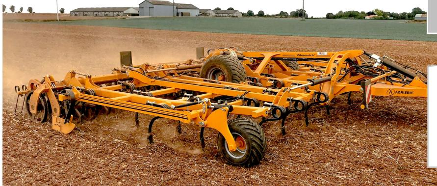
Headland manoeuvres are carried out by turning on the axle between the 4th and 5th row of tines, which allows for a compact size and great manoeuvrability.
