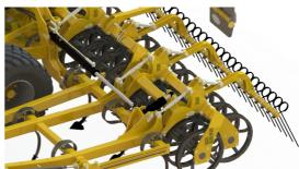
The hydraulically adjustable front **Cross-Board** kit, available on the Vibromulch, **levels the soil** before the tines and **pushes the clods** in for more efficient ploughing and **seed bed preparation.**
