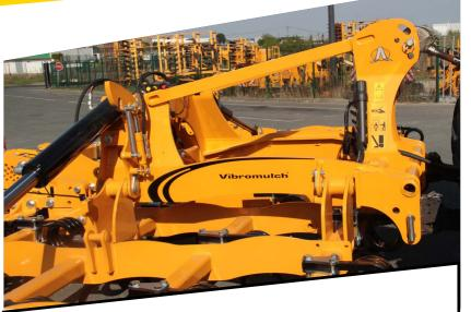
The structure is ensured by a **robust frame** whose rigidity at work is reinforced by the kinematics of the 2 folding cylinders which are held on the outside of the frame.
