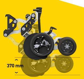
370 mm travel for a more efficient ground tracking
